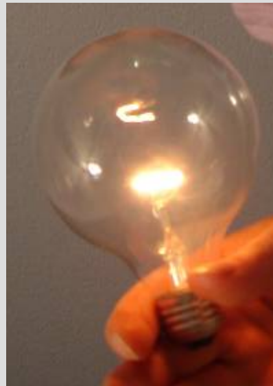
“Incandescent” Lightbulb 15 lumens per watt (5% efficient)
