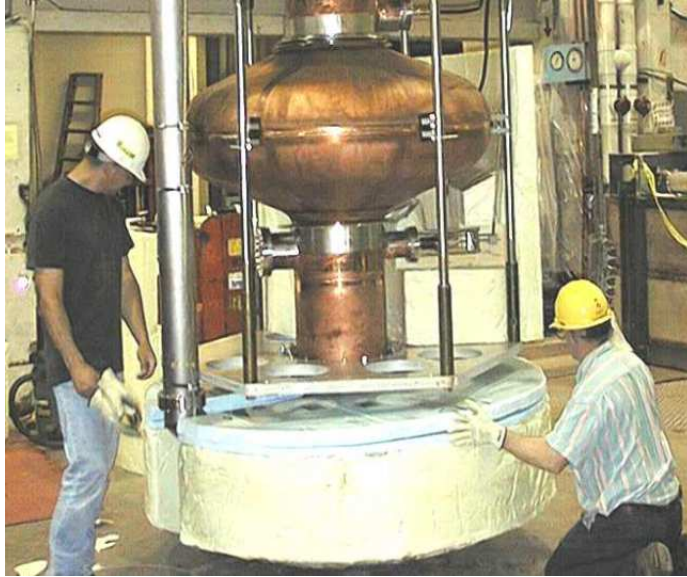
FIG. 69: (Color) 201 MHz SCRF cavity being prepared for testing at Cornell.
