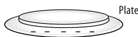
A. The Styrofoam plate is negatively charged by the wool. The electrophorus is initially electrically neutral.
