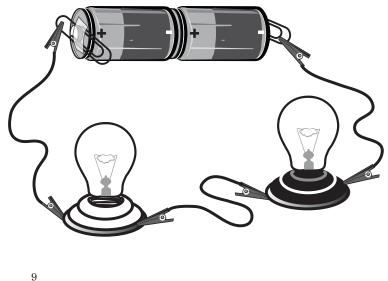
This means that less current flows through a series circuit with two bulbs than a single bulb circuit, so the light bulbs are dimmer.
