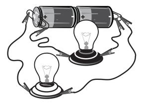
This means that overall more current flows through a parallel circuit of two bulbs than a single bulb circuit. However, the current is split between the two different paths, so each bulb gets about the same amount of current it would have if it were the only bulb in the circuit.
