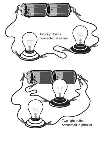
5. Use another wire to clip the free screw on the base of the second light bulb to the free end of the battery system
