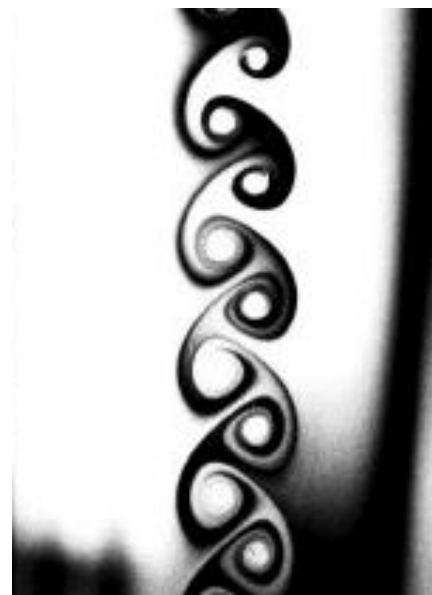
A single vortex stream behind a glass rod which punctures the film. The rod is a few mm in diameter.
