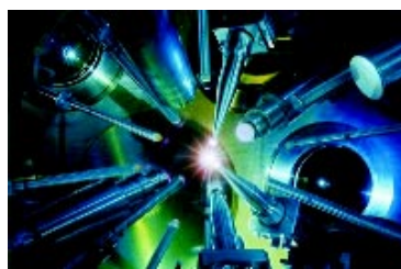
Lasers converge on a fusion target at the University of Rochester's OMEGA facility.
