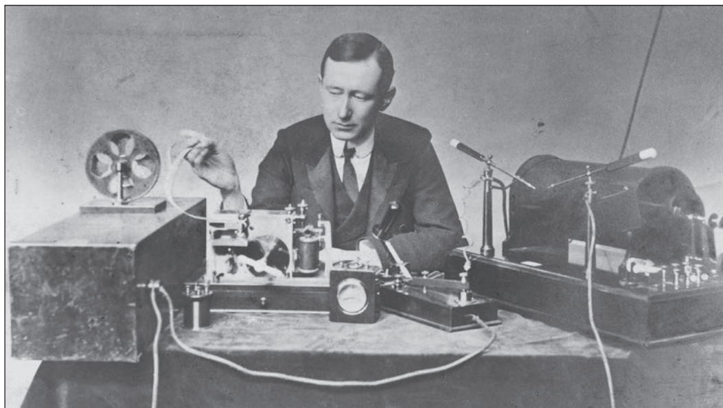
Marconi demonstrating apparatus he used in his first long distance radio transmissions in the 1890s. The transmitter is at right, the receiver with paper tape recorder at left. IMAGE: WIKIMEDIA COMMONS
