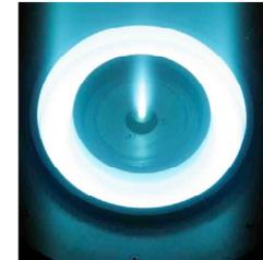
Must measure amount and divergence of ions before facility-induced collisions alter the plasma
