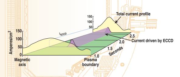
Without the ECCD, the plasma current would normally "shrink" toward the magnetic axis. Off-axis current driven by ECCD slows this evolution and can maintain a nearly steady current profile with the maximum value away from the axis, favorable for high fusion performance and bootstrap current.
