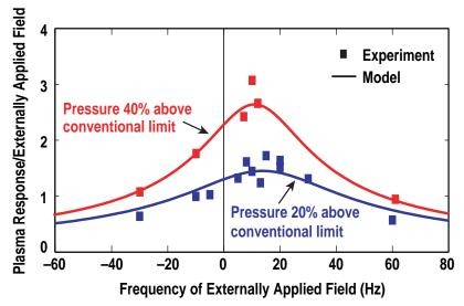
The amplitude of the plasma response peaks when the externally applied field rotates in the direction of the plasma rotation. The plasma rotation is ~6000 Hz, much faster than the mode.
