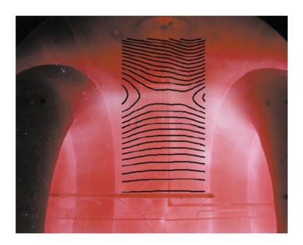
Measurement of magnetic field lines undergoing reconnection in the MRX experiment, Princeton University.
