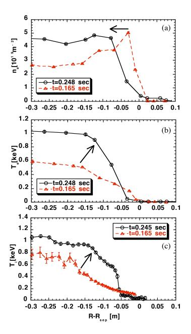
Figure 2 – Changes in the profiles of (a) electron density  $(n_e)$ ; (b) electron temperature  $(T_e)$ ; and (c) ion temperature  $(T_i)$ . The quantities are plotted against the distance from the outer edge of the plasma determined by magnetic data. The density increased mainly in the interior of the plasma, whereas the temperatures increased substantially near the edge during the enhanced H-mode phase, and the width of the steep gradient region also increased.
