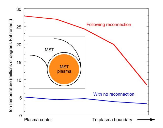
Shown here is the ion temperature measured across two MST plasmas, one in which reconnection is suppressed at all times (blue line) and one in which reconnection is utilized to strongly heat the ions (red line). The MST device and plasma are donut-shaped with a circular vertical cross section, as partially illustrated in the inset cartoon.
