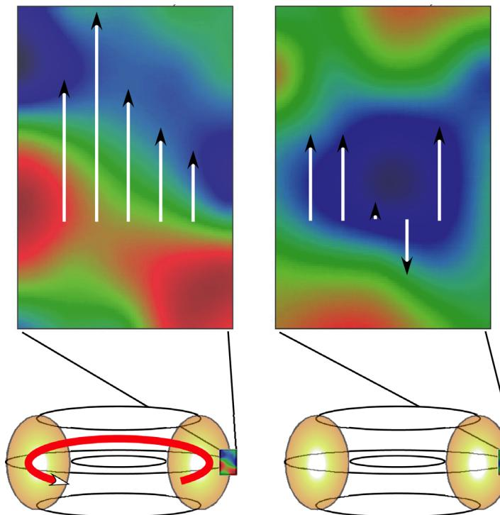
A rapidly spinning plasma, shown on left exhibits a much different turbulence flow pattern, indicated by white arrows, than the slowly rotating plasma on right. The arrows are superimposed on images of turbulence eddies measured with Beam Emission Spectroscopy. Movies of this turbulence can be viewed at: [http://fusion.gat.com/DIII-D/images/6/6d/BES\\_2shots\\_edge.mov](http://fusion.gat.com/DIII-D/images/6/6d/BES_2shots_edge.mov)
