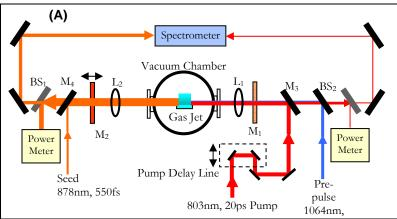
Figure1: Schematic illustrations ofthe experimental setup and method: (A) Experimental setup. Dichroic mirror  $M_1$ has high reflectivity for seed, high transmission for pump and prepulse. And dichroic mirror M2 has high reflectivity for pump, and high transmission for seed and prepulse; and (B) An illustration of input pulse amplification and compression in plasma.
