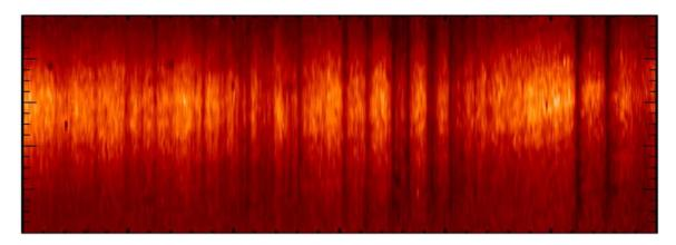
Figure: Transmission through iron heated to 1.8 million degrees. The brighter parts of the image correspond to photon energies with higher transmission, or lower opacity. The dark lines are absorption by the discrete transitions prescribed by quantum mechanics.
