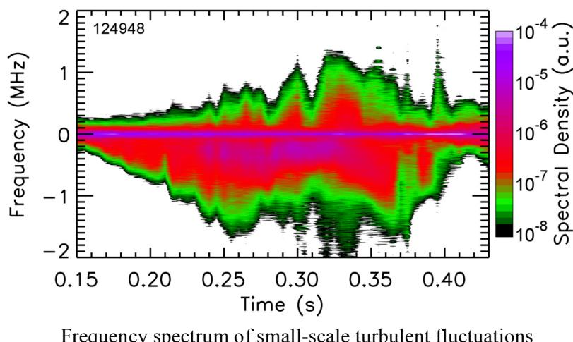
Until recently, there was no direct proof of the existence of this turbulence. Fortunately, new experiments on NSTX plasmas have detected this type of turbulent fluctuations using an advanced microwave scattering system [1]. An example is illustrated in the attached figure, showing the time evolution of the frequency spectrum of turbulent eddies with a size of approximately 2 mm. That the
