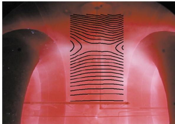
Figure 1. Magnetic reconnection seen in MRX: Oppositely directed field lines (measured) merge and reconnect.
