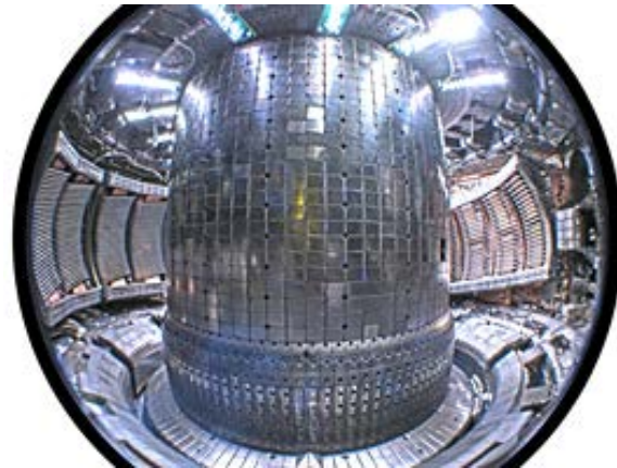
Figure 1: If these walls could talk – the tiled walls inside the Alcator C-Mod tokamak, that is - they might say they've been scarred by sudden disruptions in the hydrogen fuel that periodically impacts them. MIT researchers are discovering ways to spread out the focused energy from these disruptions so that the vessel walls are not damaged. (Photo: M. Garrett)
