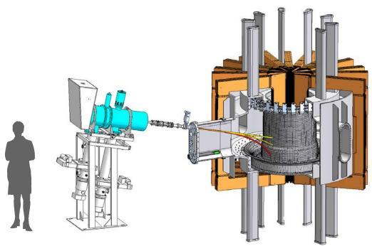
Figure 1: A small linear accelerator (left; cyan colored) injects a beam of energetic ions into the Alcator C-Mod tokamak (right). The ions are magnetically steered with tokamak magnets (copper colored) to different locations (yellow, orange, and red colored) on the wall. Analyzing the nuclear reaction products with small detectors (green colored) induced by the beam provides crucial information about the materials inside the device.
