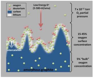
The lithium coating on graphite, which appears mountainous in this graphic done at microscopic scale, provides the perfect setting for oxygen to control the hot deuterium plasma. Reference: C.N. Taylor, et al., "The role of oxygen in retaining deuterium in lithiated graphite", J. Appl. Phys., submitted 2013.
