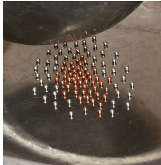
Figure 2: The flexibility of the gravity crystal concept allows exploration of the same physics that governs oxygen-carbon stratification within cool white dwarf stars. This can be observed by mixing different mass spheres (copper and aluminum) in “Alina’s bowl,” a shallow stainless-steel kitchen mixing bowl. Once voltage is applied, the heavier copper balls “sink” to the bowl center and separate from the lighter aluminum balls. (Credit: Alexander Bataller)
