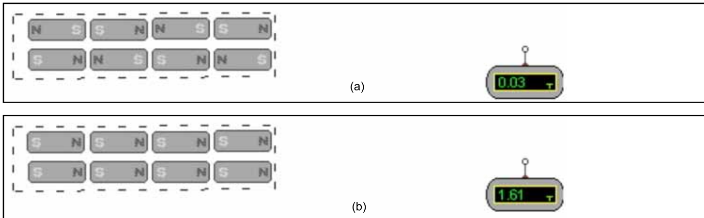
Figure 8. A computer simulation that shows the strength of the magnetic field at a position external to a group of magnets. (a) Four magnets with North Poles oriented one way, and four with South Poles oriented the same way. The reading on the field meter has a very low value. (b) Eight magnets with North Poles oriented the same way. The reading on the field meter has a much higher value.
