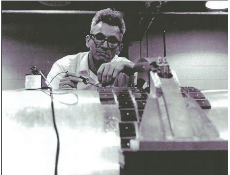
Joe Weber after installing new gold plated quartz piezoelectric strain gauges
