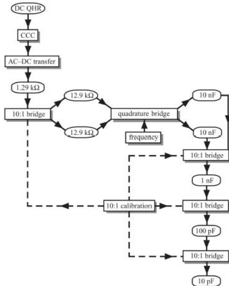
Figure 5.1: Traceability chain for the realisation of capacitance (at 10 pF – 100 pF level)
