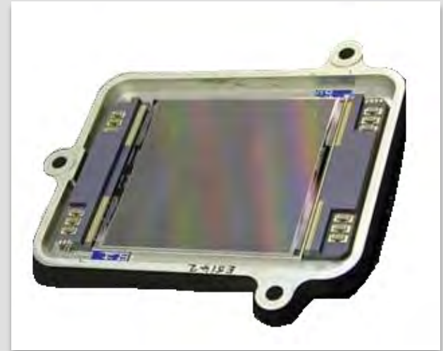
HMI and AIA use 4096 x 4096 CCDs built by e2v in England.
